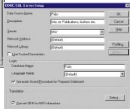
Fig 13 (left) Next, from within Access you can elect to link to a table via an ODBC connection
